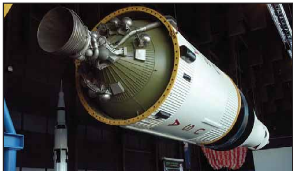
A Saturn 5 Apollo Rocket hangs in the main building of the Space Center. This picture shows the second stage of the rocket with the larger first stage hanging behind. The Apollo capsule itself is the the small white tip of this massive machine.
